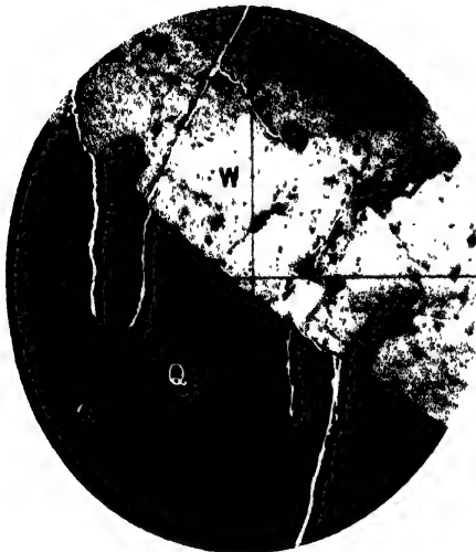
FIG. 3. PYRITE VEINLETS IN QUARTZ (Q) AND WOLFRAM (W). ( \times 54 ).
